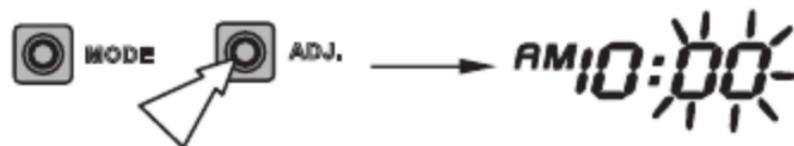
7. To end the clock adjustment, press both the MODE and ADJUST buttons at the same time. The display will stop flashing automatically. The adjustment will be cancelled if any button is not pressed within approximately ten seconds
