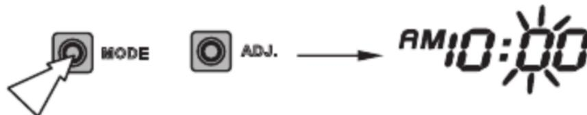
6. To set the minute display, press the ADJUST button until it displays the correct "minute" time
