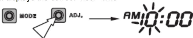
5. To change the minute display, press the MODE button until the "minute" digits begin flashing
