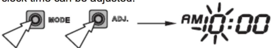
4. To set the hour display, press the ADJUST button until it displays the correct "hour" time
